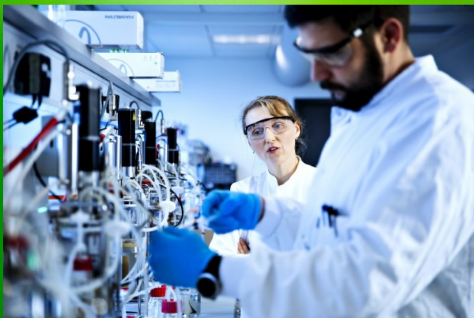
Figure 3: PHERA Technical Manager and BioPhero Chief Scientific Officer Irina Borodina at the company’s small bioreactors used to test various yeast strains optimised for the production of insect pheromones. (Image: BioPhero, Colorange Photography, Thomas Steen Sørensen).
